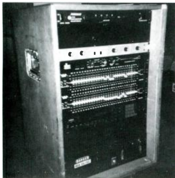
Figure 3. Two equalizer settings of aligned monitors. Because of the smoothness of an aligned system, the top eq is set to remove the peaks common to the Shure SM-57 while the bottom eq is set for a SM-58. Notice that the presence peak had to be removed from the SM-58.
