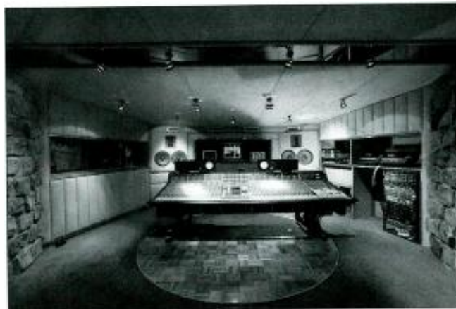
Figure 1. The console mounted on a turntable so it can do multiple duty.
